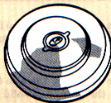
5 Indicator Turned To "ARMED" Position After Laying Mine.
