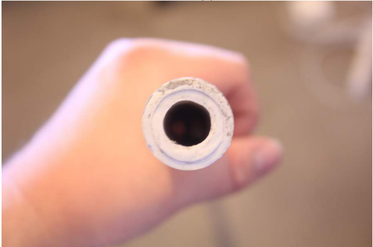
PVC bow made from two PVC pipes, one inside the other
