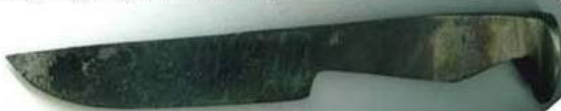
Heat treated - logo stamped on blade, oil quench for high carbon water for med carbon
