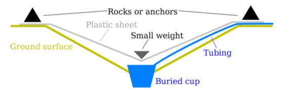
Solar Still Design. Make sure the plastic sheet overlaps the edge of the hole enough to lay the rocks.
